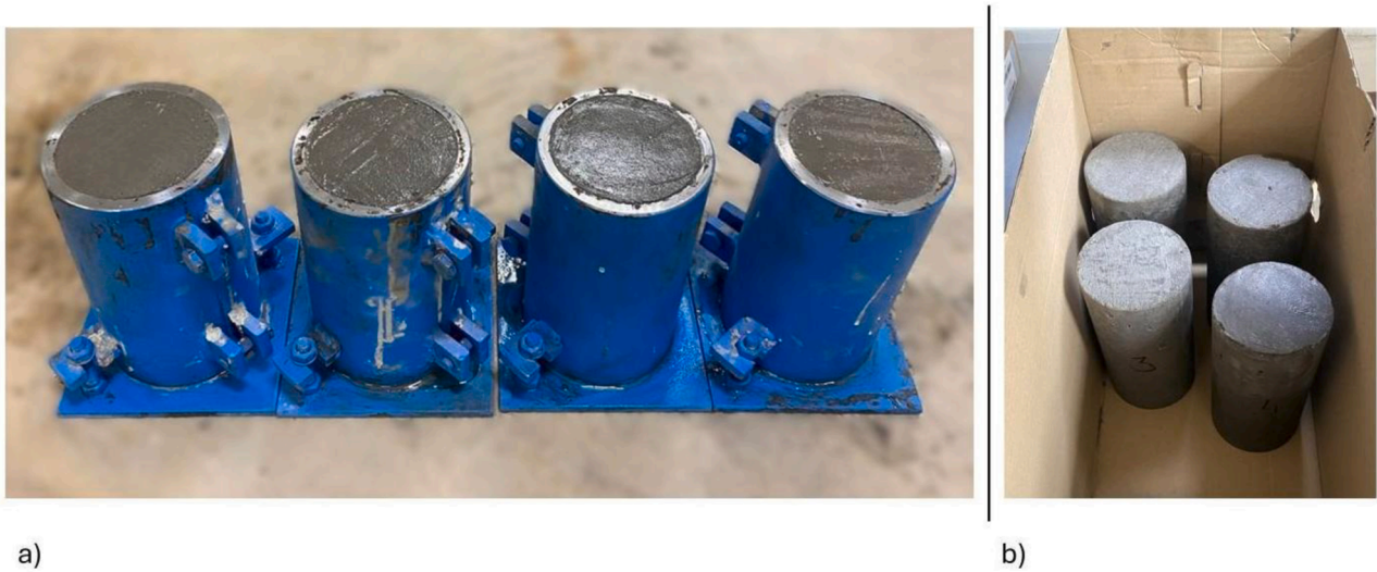
Fig. 3. a) Freshly cast stabsoil specimens in cylindrical molds; b) curing of stabsoil specimens.
